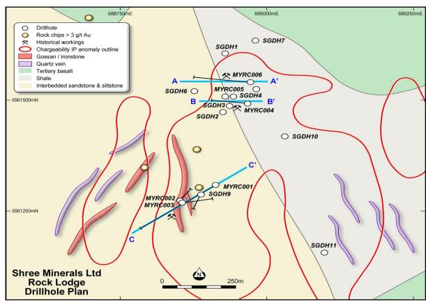
**Figure 5.** Historical exploration summary diagram showing the main geological features of the Rock Lodge prospect. Past drill hole locations, anomalous rock chip sampling and IP chargeability anomalies are also illustrated.
