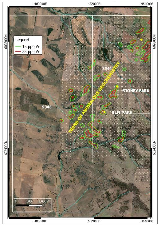
Figure 3. Historical soil geochemistry contours showing a distinctive north-easterly south westerly trend of the contours. Also shown is the aerial extent of the soil sampling survey (white stippling), with 70% of EL9346 remaining unsampled.
