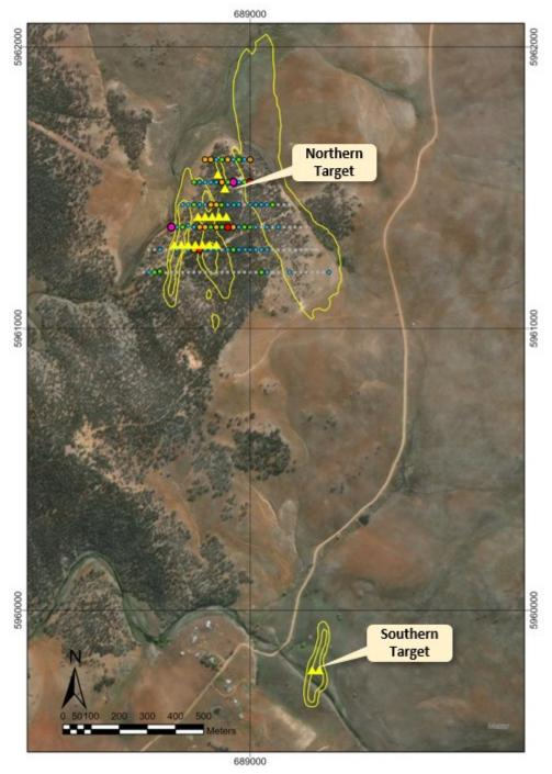
Figure 4: Rock Lodge prospect showing proposed RC holes (yellow triangles) testing IP chargeability anomalies (yellow polygons) with coincident gold soil anomaly (orange >50ppb Au, red >100ppb Au, magenta >250ppb Au)
