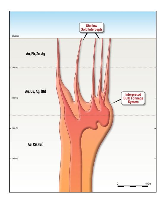
Figure 8 : Diagrammatic figure of the Intrusion Related Gold System model at Rock Lodge prospect
