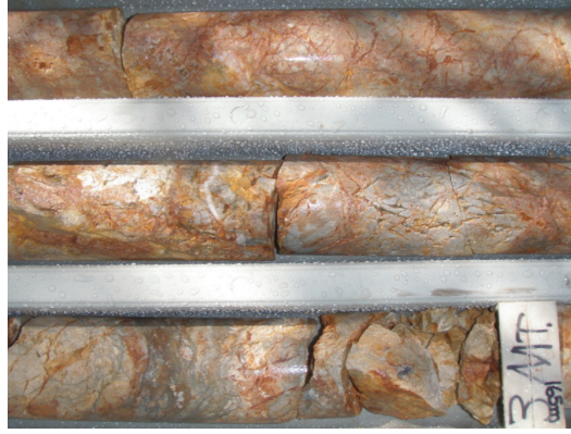
Plate 2: Typical stockwork veining in drill hole SCDDH5
