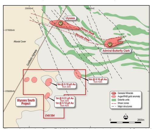
**Figure 6**. Location Plan: E40/384 (Ulysses) showing location of Genesis Minerals Ulysses and Admiral-Butterfly resources. Gold mineralisation is controlled by dolerite units and northwest trending faults
