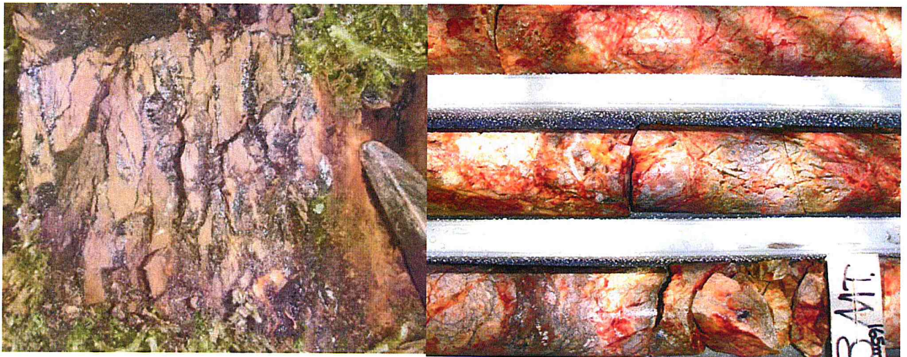
Typical stockwork veining in SCDDH5 ~165m (3m @ 1.29g/t AU)
