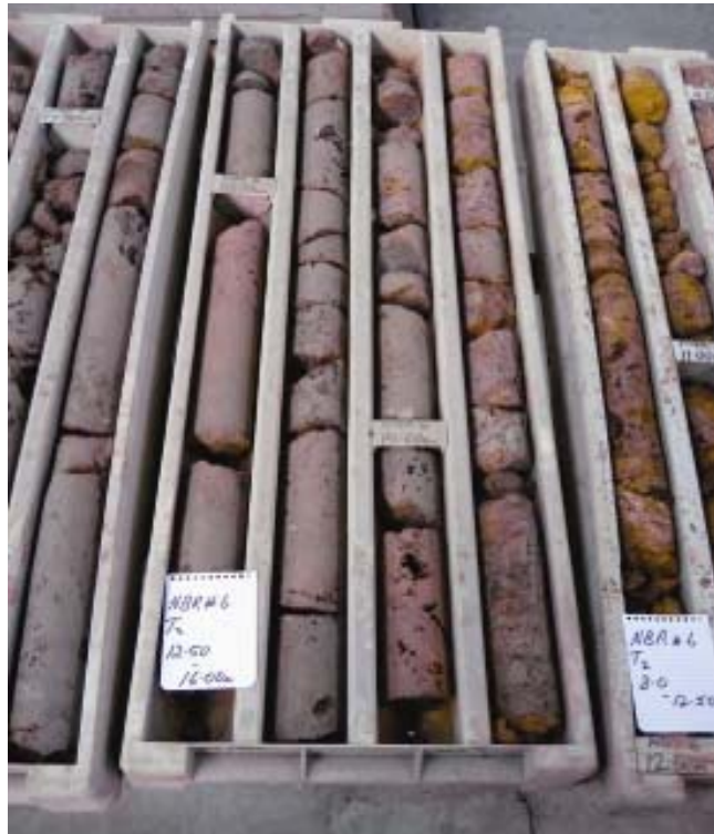
Plate 2: Goethitic hematite core from drillhole NBR-6
