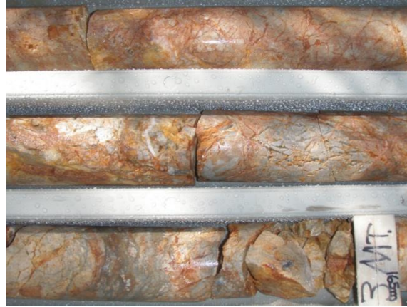
Plate 1: Stockwork with ferruginous veins in drill core – Davie Prospect
