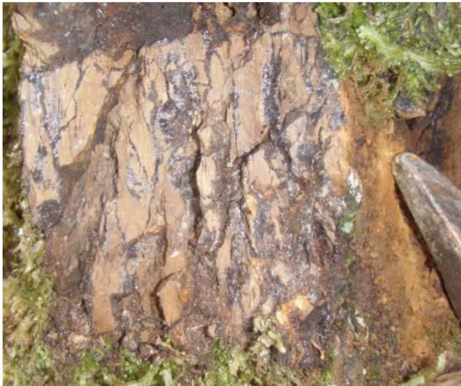
Iron oxidised stockwork veining near the Davie Adit (<0.01g/t Au).
