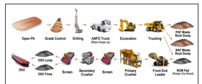
Figure 2: NBR DSO Flowchart
