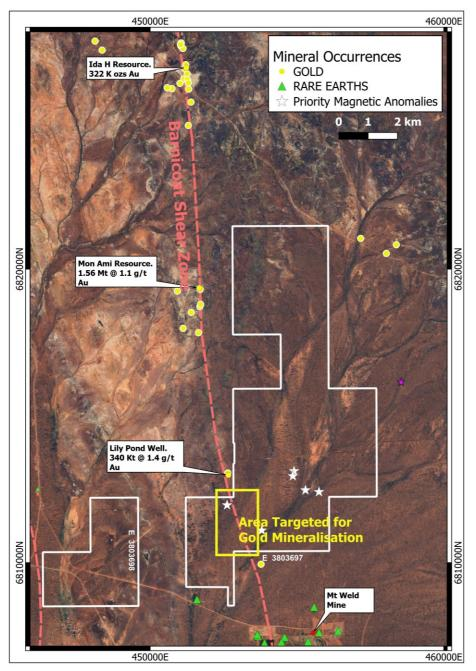
Figure 1 – Satellite image showing location of proposed drilling relative to the north-south trending Barnicoat Shear Zone and related gold resources.
