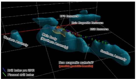
Figure 5: 3D Magnetic Inversion Study (Source: SHH)
