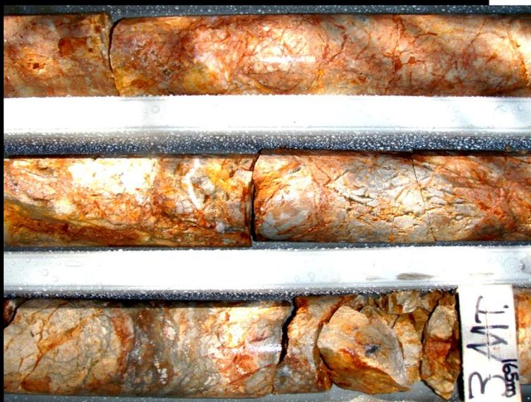
Stockwork veining in drillhole SCDDH5
