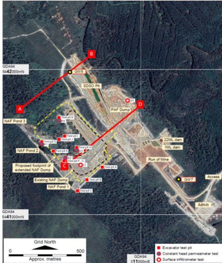
Figure 5. Existing NAF Dump and its proposed extended footprint, excavator test pit and permeability test locations (7 – 8 May 2019), and hydrogeological section lines A – B and C – D. (Source for base image: Google Earth, 6 December 2018)
