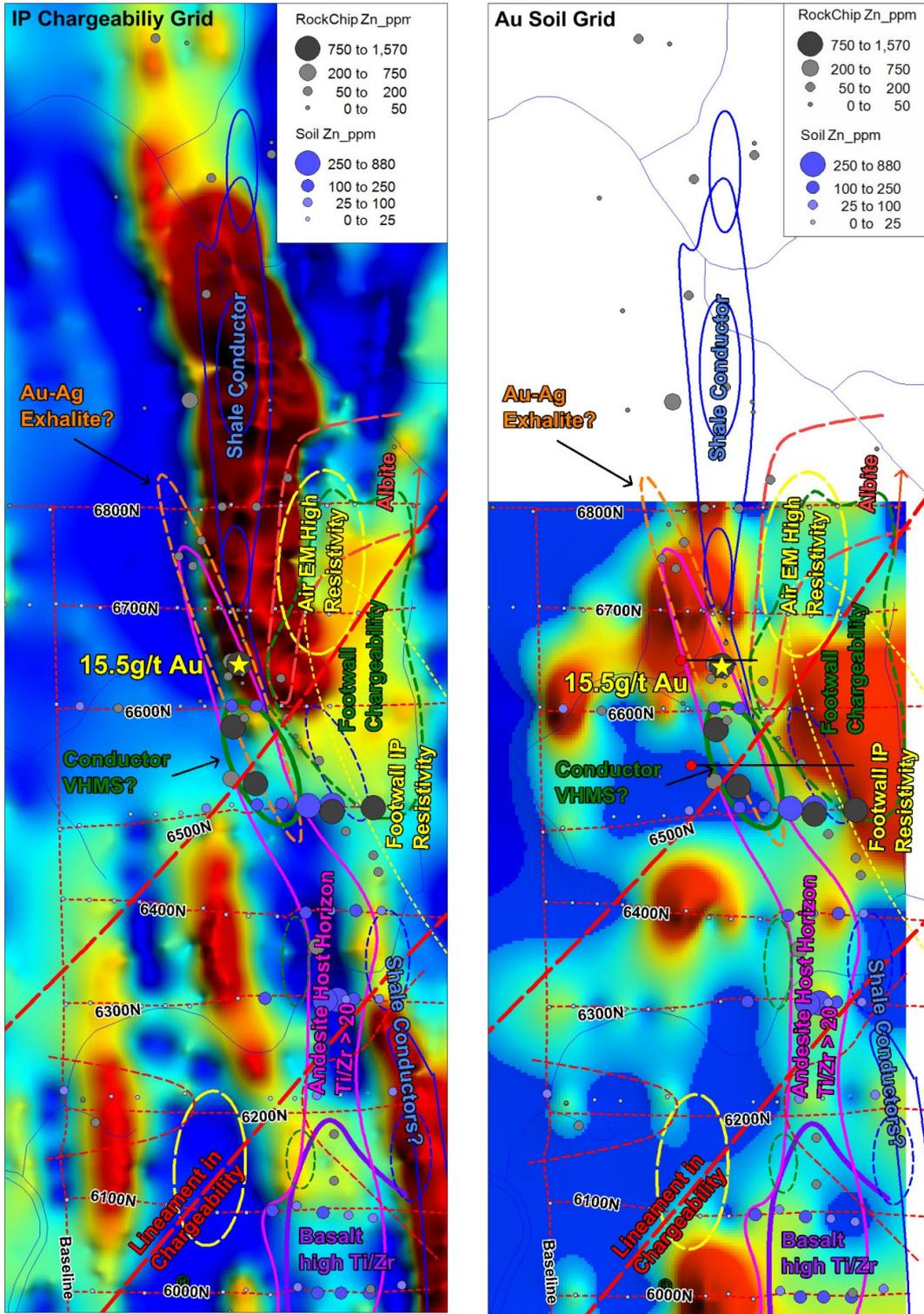
VHMS prospectivity map for the northern half of the Clark River Grid showing Zn in rock chip and soil thematic and recommended drill holes over IP Chargeability grid (left) and Au in soils grid (right).
