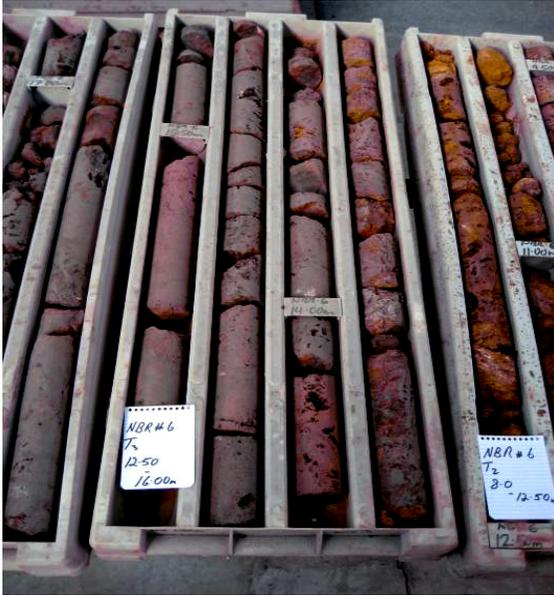
Plate 1: DSO iron ore core
