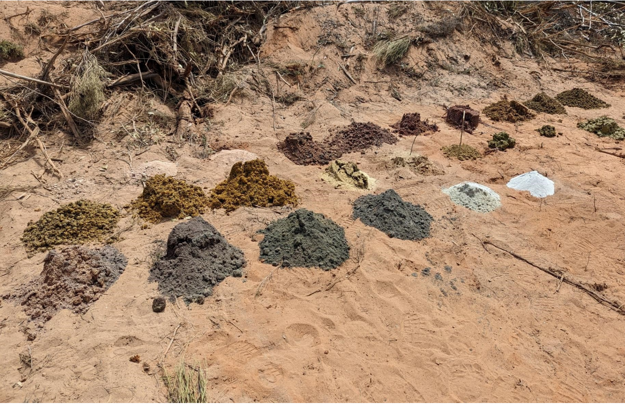
Figure 2. Samples from Aircore Drilling in progress at E63/2046.
