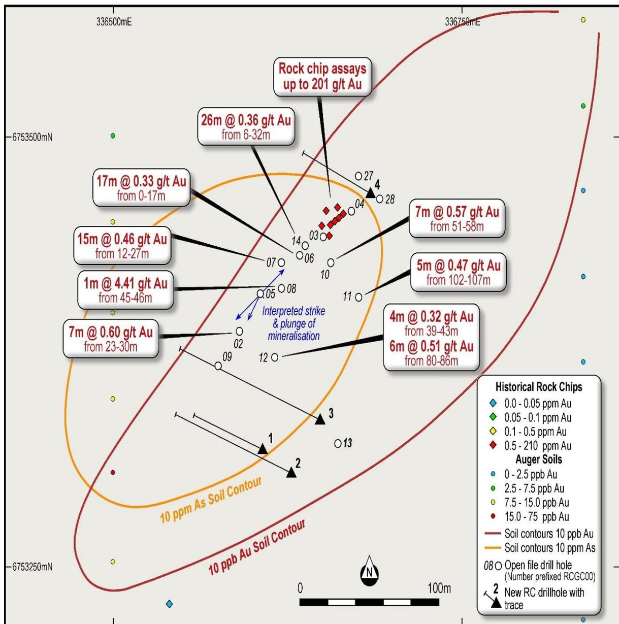
**Figure 3.** Location of the historical and the recent RC drilling at the Golden Chimney prospect. Auger soil geochemistry contours (Au, ppb and As, ppm) are also shown.
