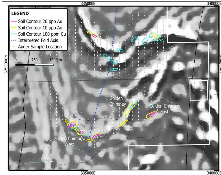
**Figure 2.** Multi-element (Au, Cu) soil contours derived from Shree's auger program. Also illustrated is the location of all auger samples and the interpreted position of the regional fold axis. The underlying image is the aerial magnetics.
