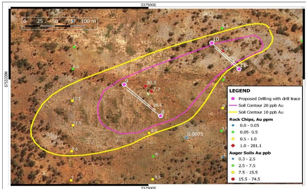
Figure 4. Location of the recently completed RC drill holes at the Golden Chimney East prospect.
