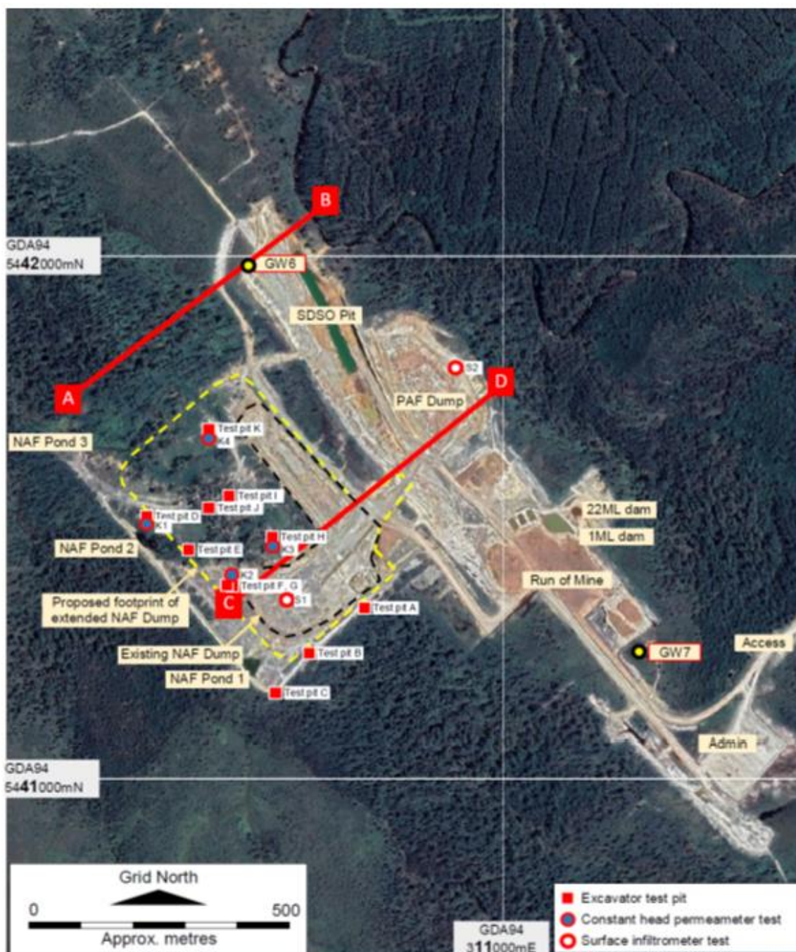
Figure 5. Existing NAF Dump and its proposed extended footprint, excavator test pit and permeability test locations (7 – 8 May 2019), and hydrogeological section lines A – B and C – D. (Source for base image: Google Earth, 6 December 2018)
