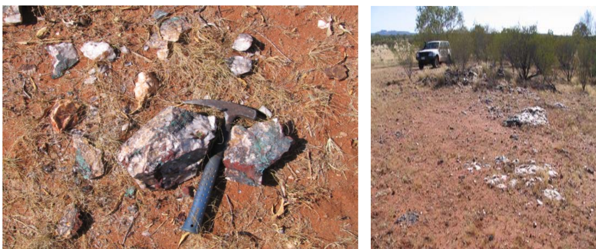
Figure 7. Malachite in gossanous veins at Bruce's Prospect; samples from here yielded 1.9g/t Au and 1.6% Cu. (563990E, 7474581N).
