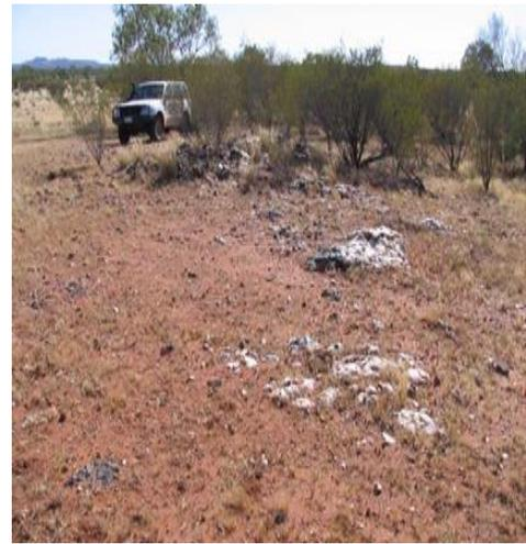
**Figure 5.** Malachite in gossanous veins at Bruce's Prospect; samples from here yielded 1.9g/t Au and 1.6% Cu.
